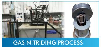
Gas nitriding is a thermochemical case hardening process used to increase wear resistance, surface hardness and fatigue life by dissolution of nitrogen and hard nitride precipitations.
