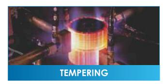
The main advantages of Tempering Process reduction in hardness & to improve the temper resistance.
