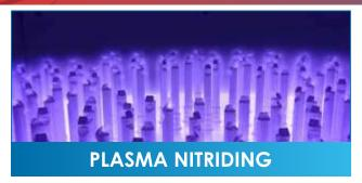
The main advantages of plasma nitriding over conventional nitriding processes are: reduced cycle time, controlled growth of the surface layer, elimination/Controlled white layer, reduced distortion, no need of finishing, pore-free surfaces and mechanical masking ...etc.
