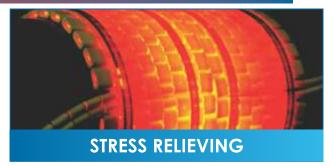
The main advantages of Stress Relieving process to minimize residual stresses in the structure thereby reducing the risk of dimensional changes during further manufacturing or before the final use of the component.
